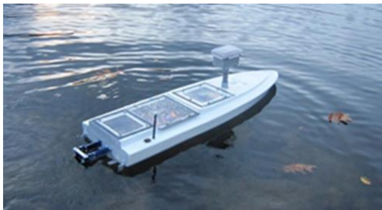
Figure 2. Image of the ASV during deployment for the Fishing Creek reservoir bathymetric study.
